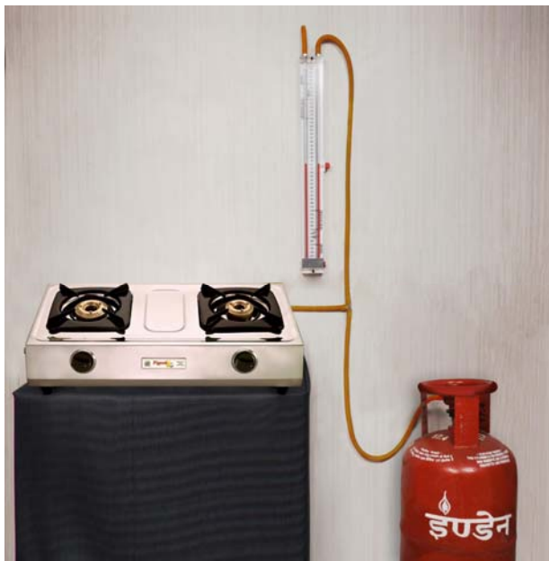
DIAGRAM NO 10: TESTING OF DOMESTIC PRESSURE REGULATOR
